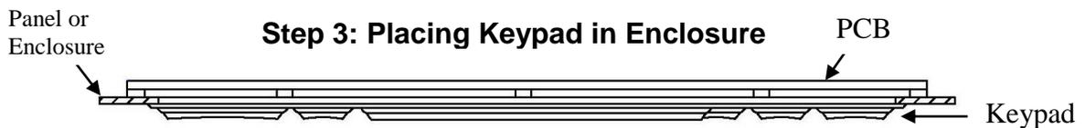
1. Put the silicone rubber keypad into place on the panel or enclosure you are using. Do not place PCB yet.
