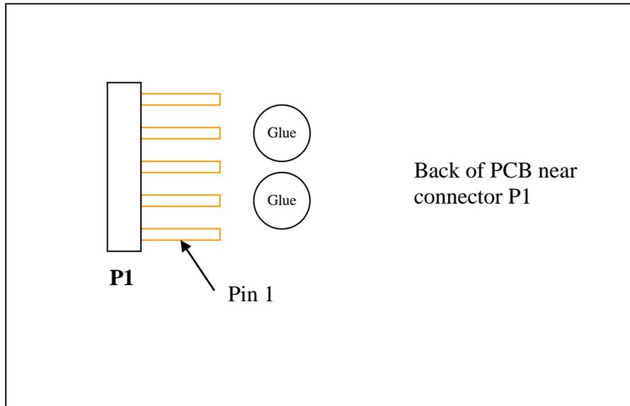
Add a dab or two of glue on the PCB just in front of the connector so that the cable header will sit on the glue when connected to the board and make itself more secure. The picture above illustrates the placement of the glue prior to the connection
