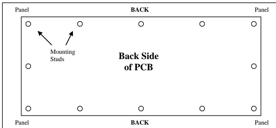
5. Tighten hex nuts until keypad is just SLIGHTLY compressed between panel and PCB. We recommend 1.5 in/lbs. of torque when tightening.
