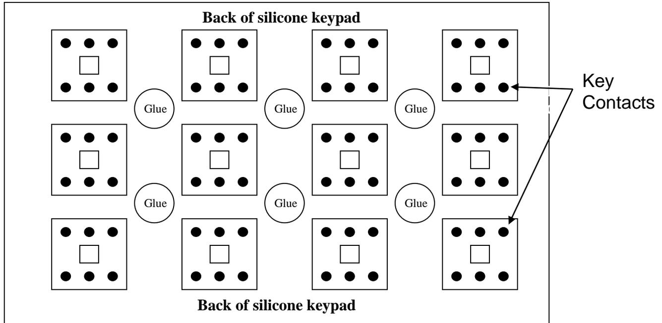
Apply silicone adhesive [iKey recommends SuperFlex by Loctite] to back side of silicone overlay (keypad). Sparingly dab glue on the middle of each key intersection across the whole keyboard as seen in this picture. Also apply to inside of center portion of HulaPoint™ pad (where the sensor/joystick lies) if OEM kit incorporates the HulaPoint™
